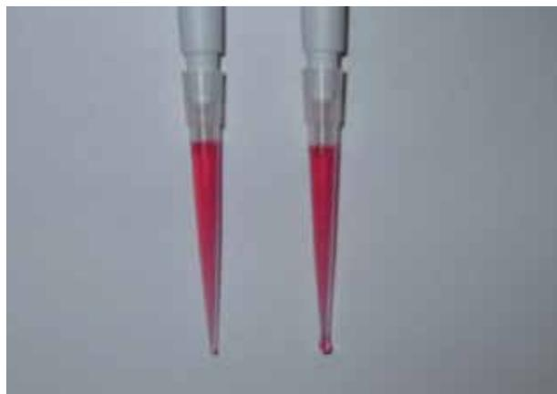
Figure 2: Evaporation causes the liquid to squeeze through the tip orifice if the tip is not pre-wetted. On the right a dry tip, and on the left a pre-wetted tip with a colored ethanol solution 15 s after the aspiration.
