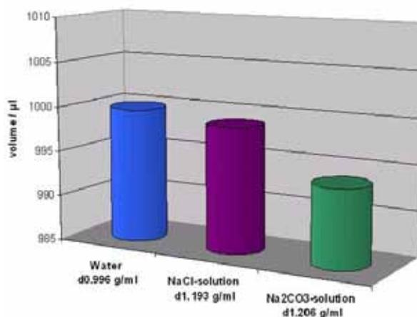
Figure 1: Effect of liquid density on the delivery volume. Differences between water, saturated NaCl solution and 20 w-% Na<sub>2</sub>CO<sub>3</sub> solution. Individual measurement variation shown along with the average value of test results.
